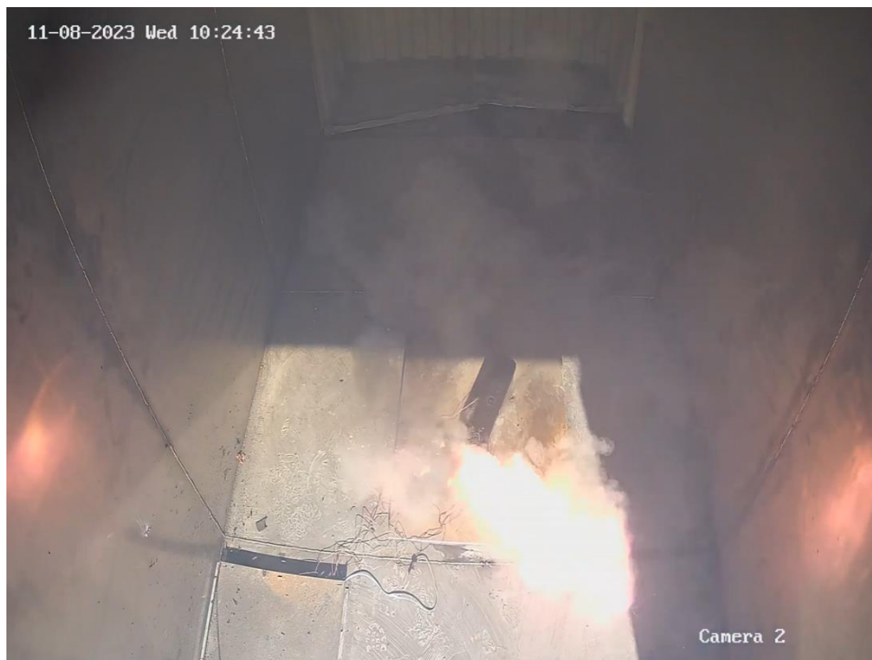
Figure 68. Cell to cell propagation within the battery.
