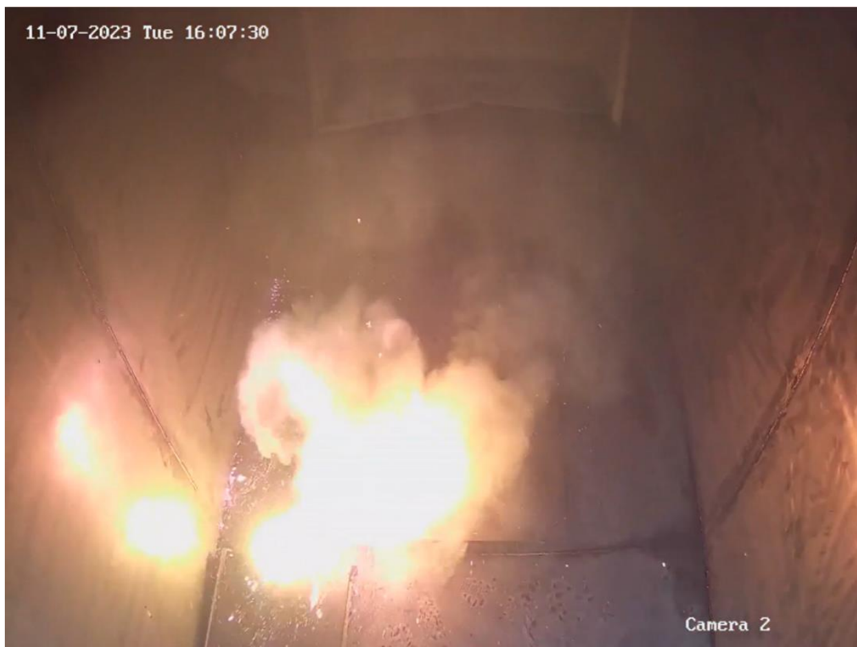
Figure 46. The E-Bike battery experiencing propagation from cell to cell.
