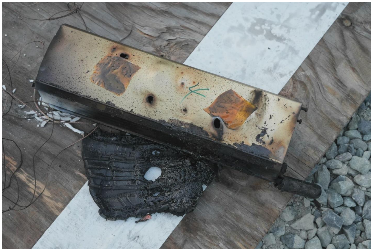
Figure 108. View of E-Bike case with visible holes post control test.
