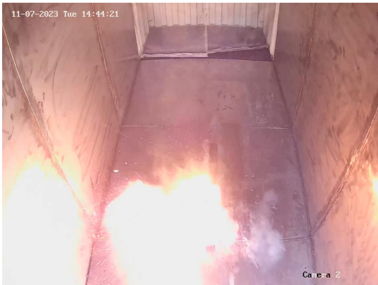
Figure 82. View of thermal runaway before the application of FCL FSS.
