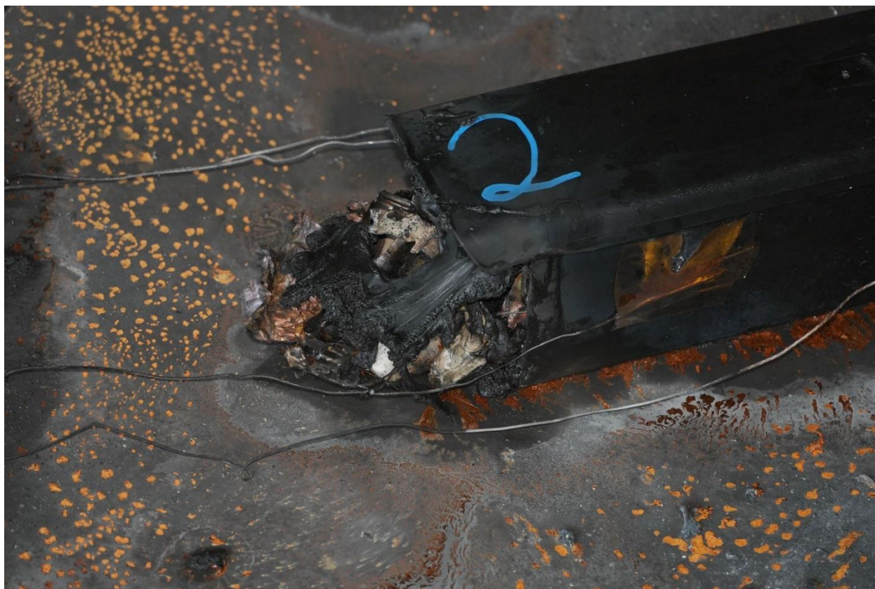
Figure 59. Close-up photo of the E-Bike battery after the third application of water.
