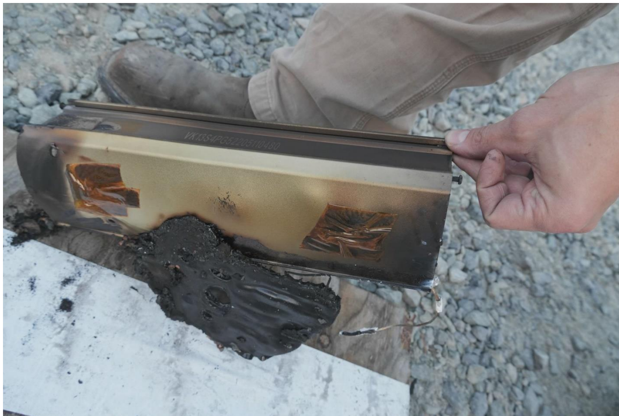
Figure 110. Dents visible on the opposite side of the metal case.
