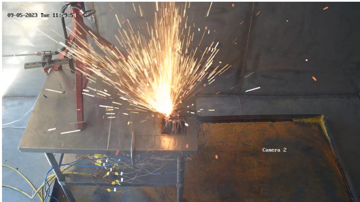
Figure 11. Fifth cell undergoing thermal runaway.
