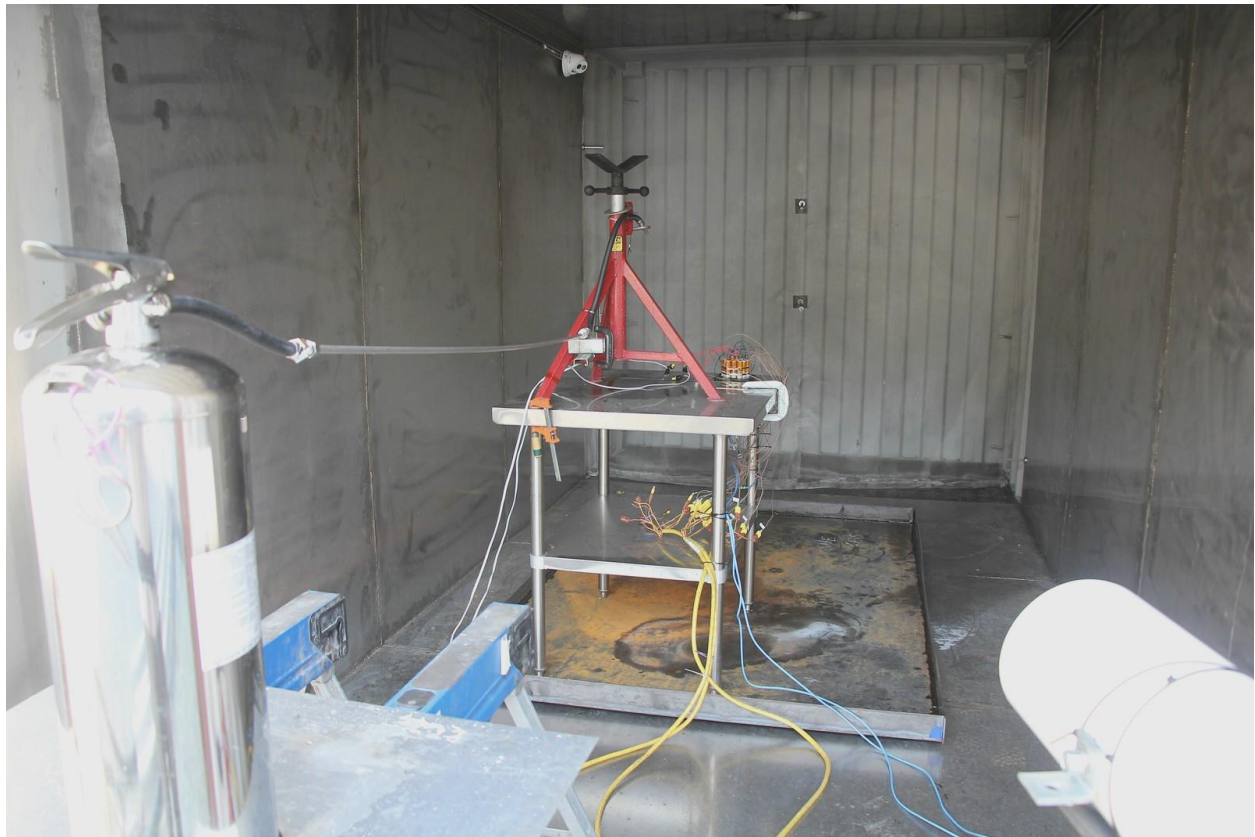
Figure 2. Test setup overview, looking inward.
