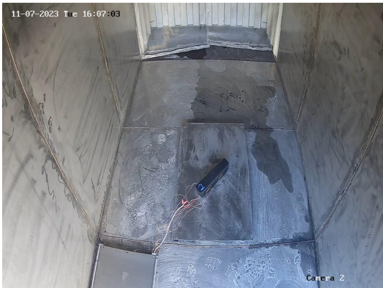
Figure 43. Right before the first cell experienced thermal runaway.
