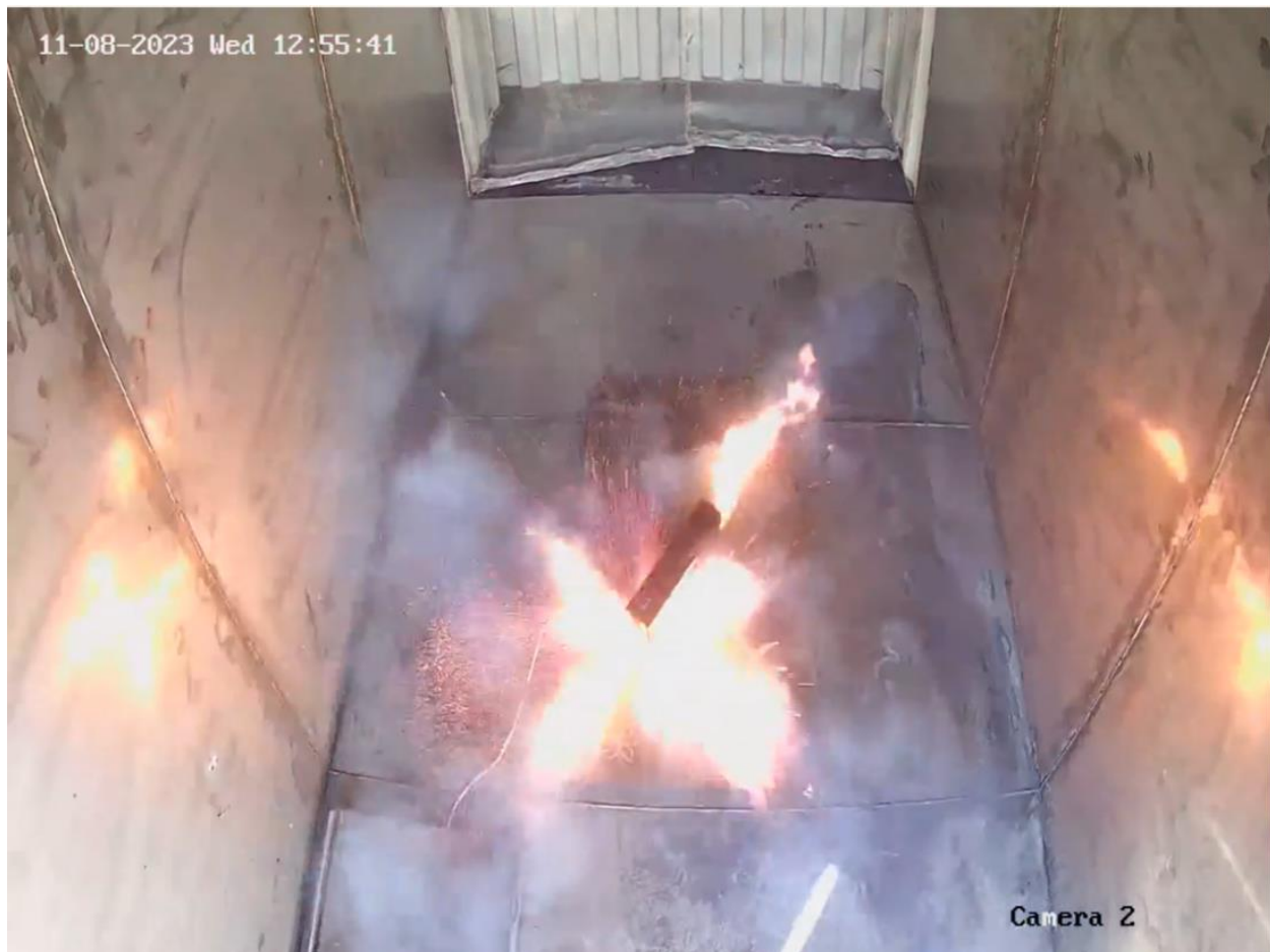
Figure 93. View of thermal runaway.
