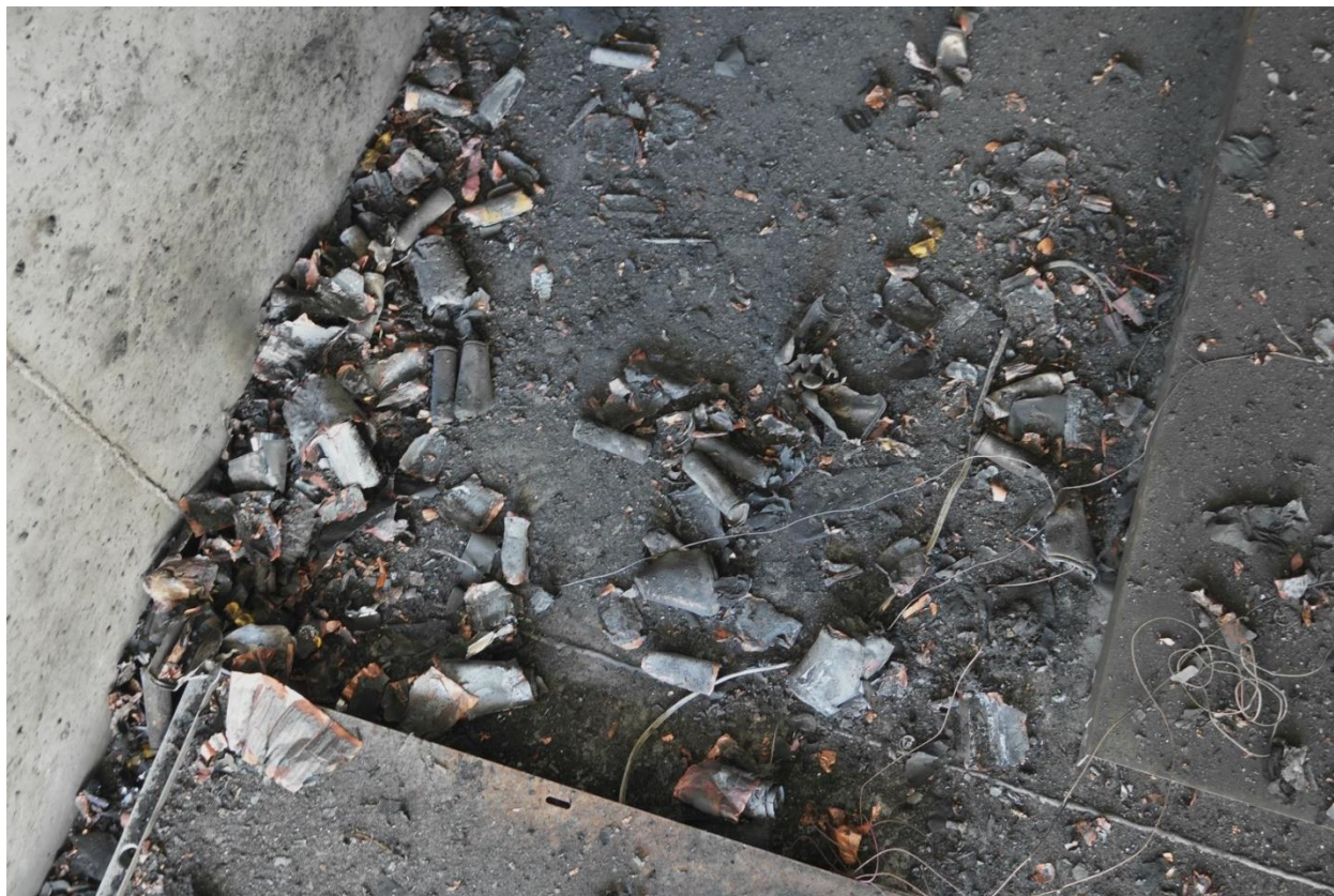
Figure 105. Debris from the inside of the E-Bike battery.
