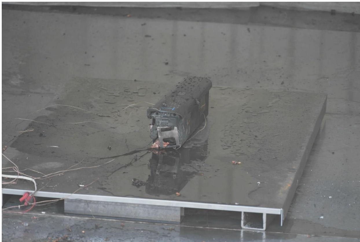
Figure 87. Photo of E-Bike battery post application of FCL FSS as an extinguishing agent.
