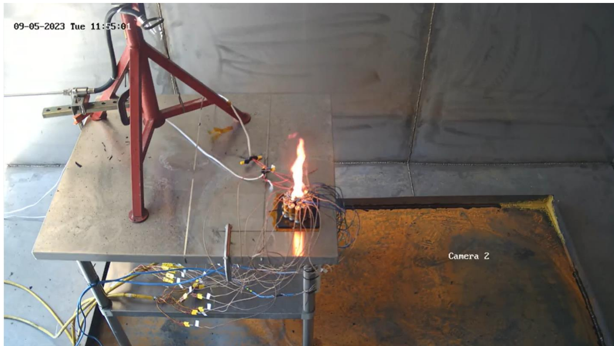
Figure 10. Small flame that heated up adjacent cells.
