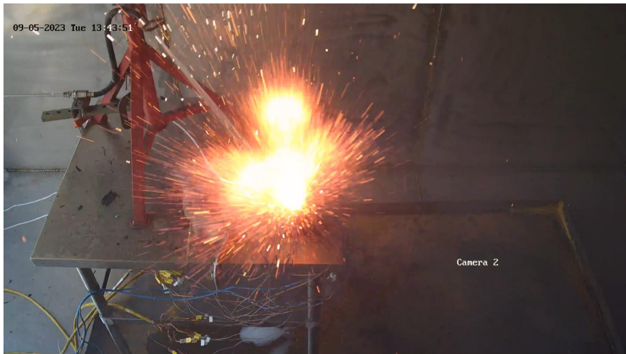
Figure 23. Second time F500 is sprayed on the cluster during propagation.
