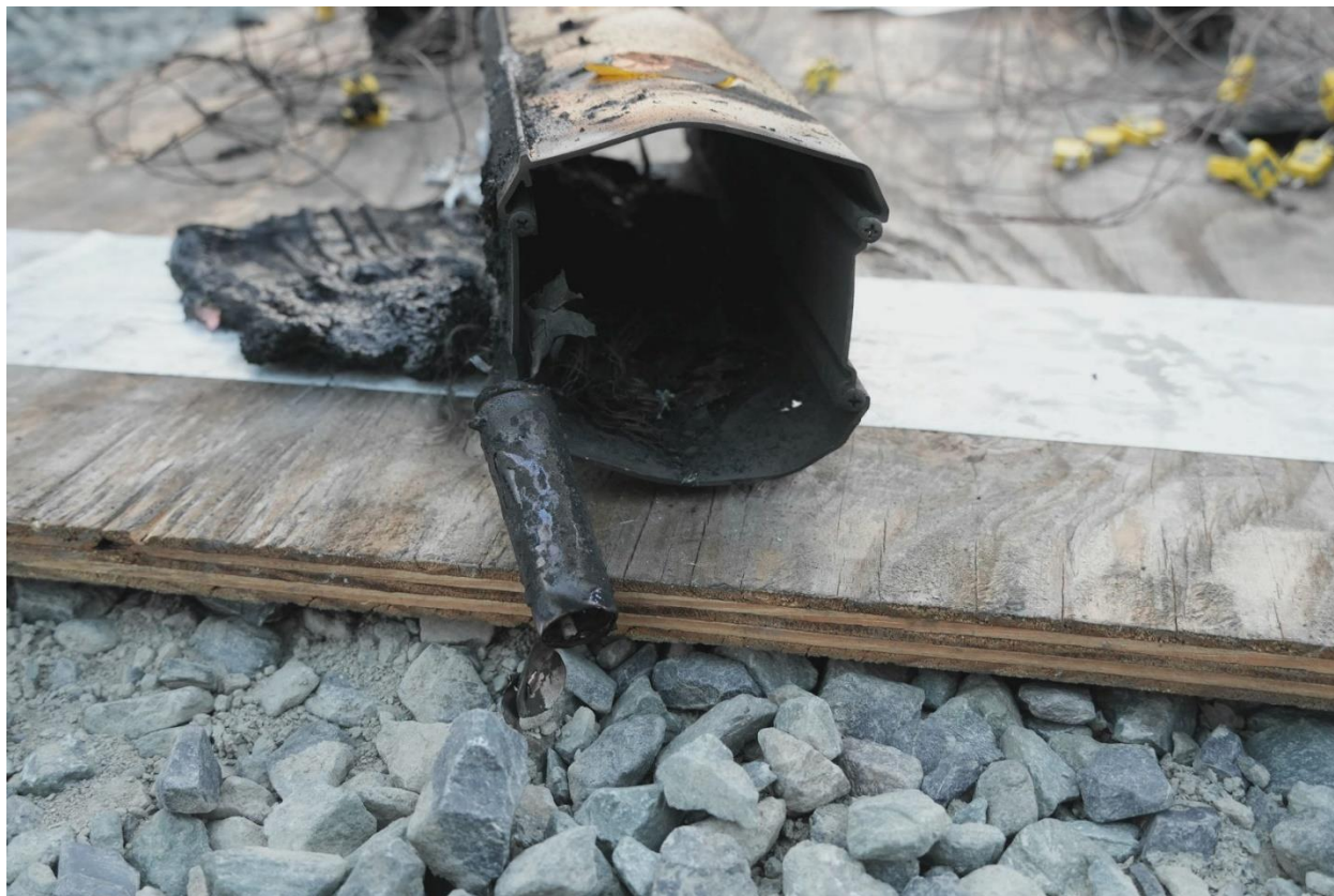
Figure 109. View of E-Bike case with no cells visible within the battery.
