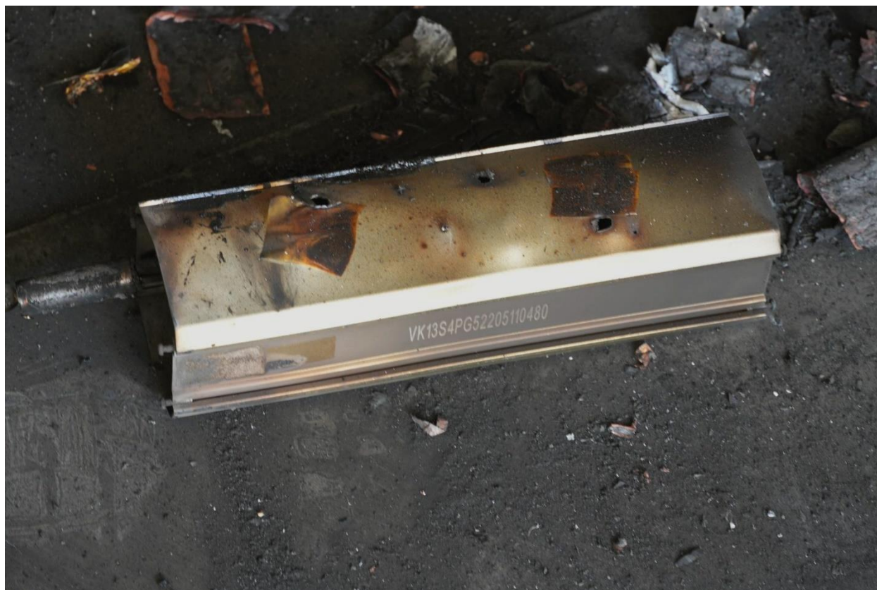
Figure 106. Metal case of the battery with visible holes.
