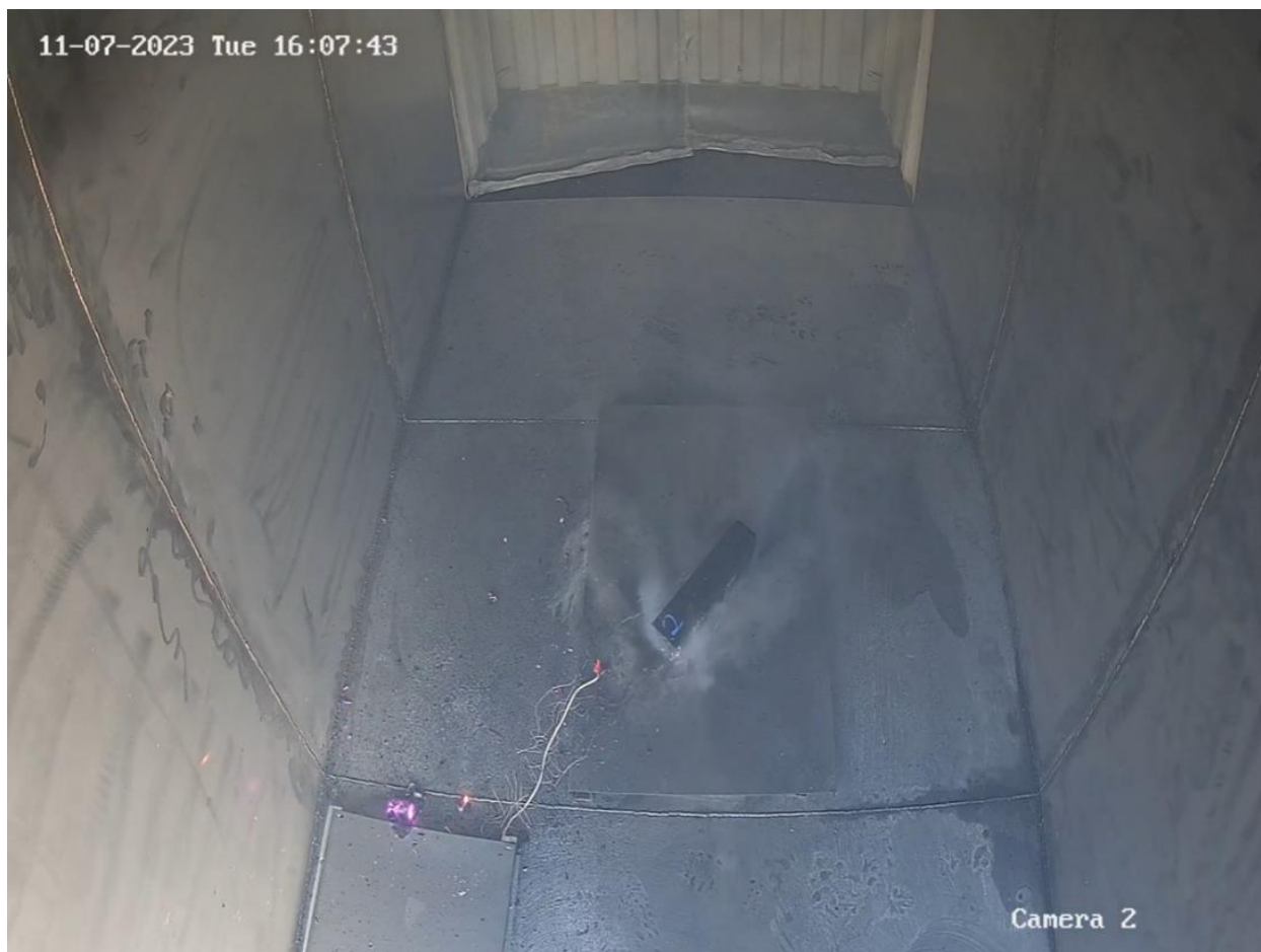
Figure 49. Battery continues to smoke and off gas after water was applied.
