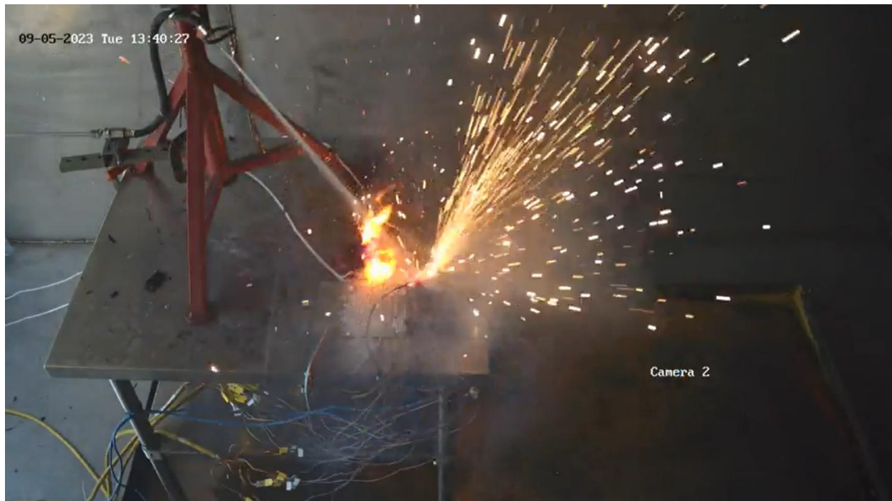
Figure 21. F500 is sprayed on the cell cluster.
