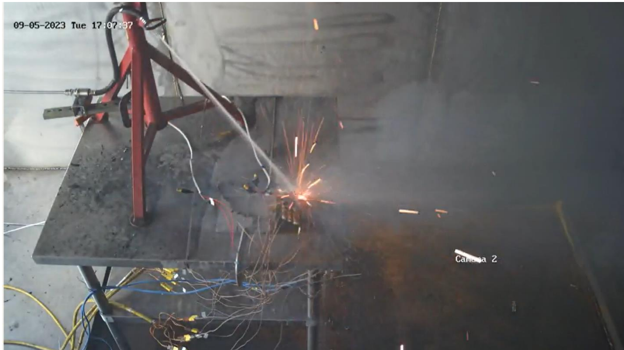
Figure 27. FCL FSS was applied after five cells were experiencing thermal runaway.
