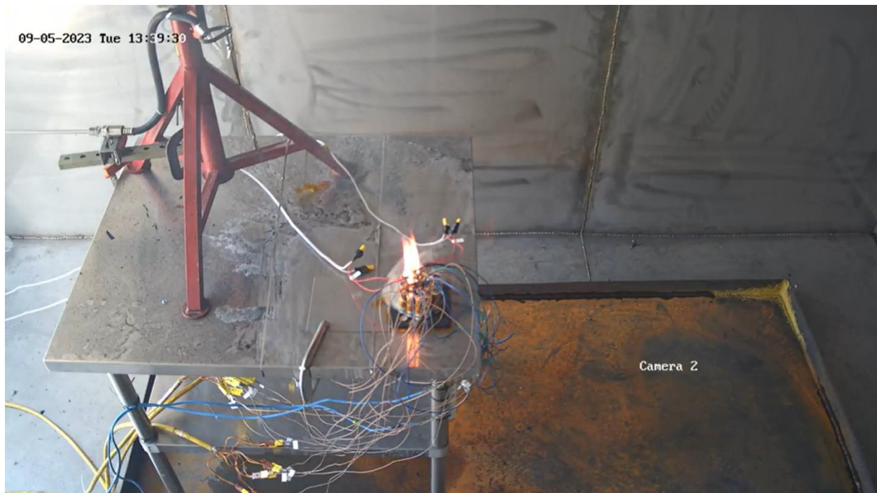
Figure 20. Small flame and off gassing.
