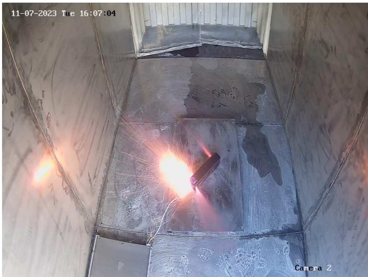
Figure 44. First cell experienced thermal runaway.
