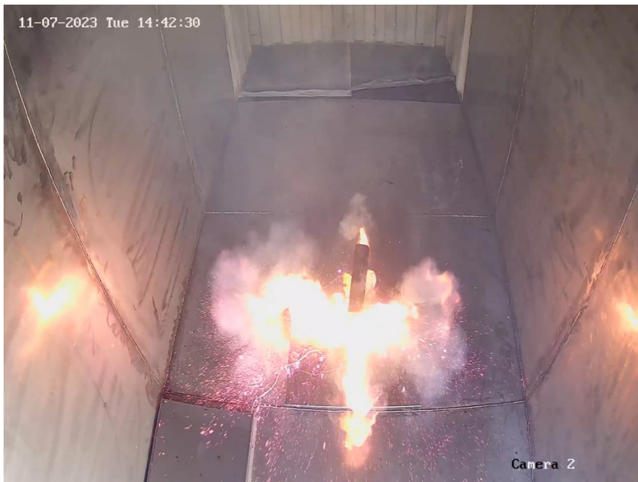
Figure 81. Propagation to other cells within the E-Bike battery.
