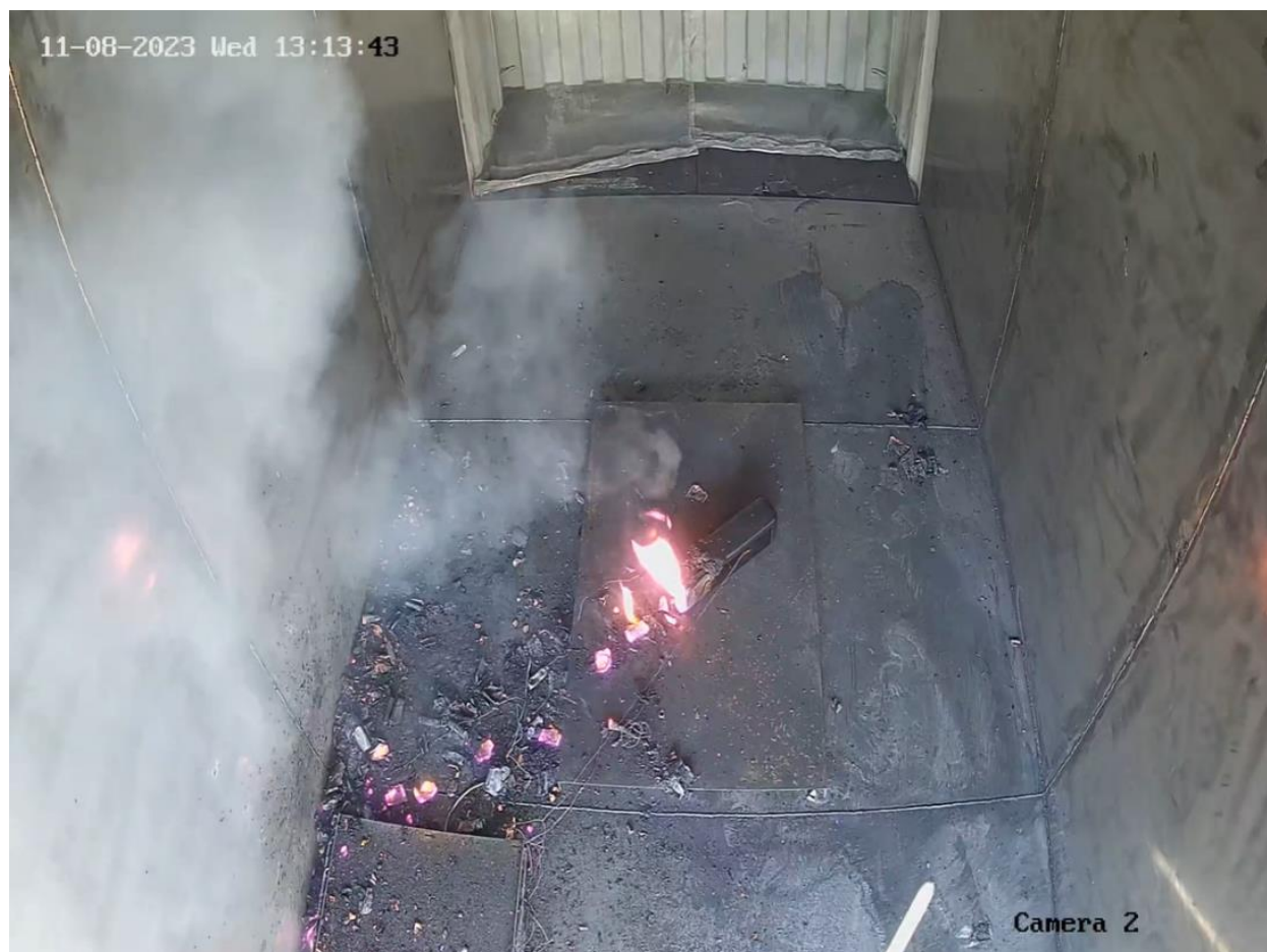
Figure 95. Progression photo of control battery with sustained flame.
