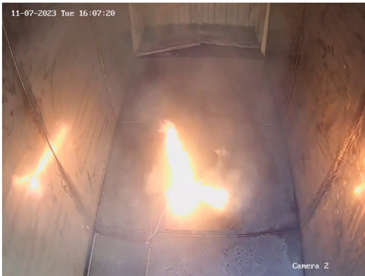
Figure 45. Progression view of multiple cells experiencing thermal runaway.
