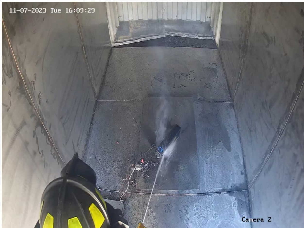
Figure 52. Water applied after reignition.
