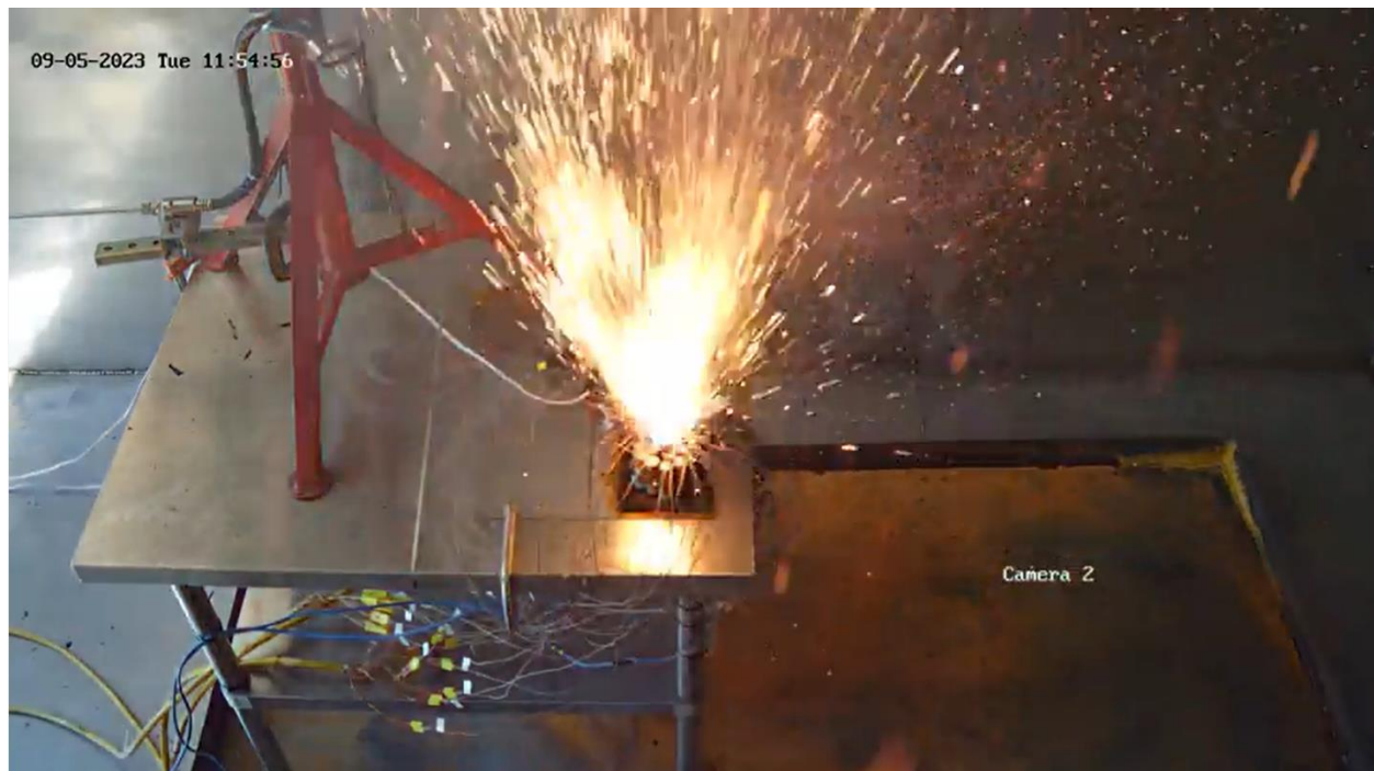
Figure 9. First cell undergoing thermal runaway, t=00:00.
