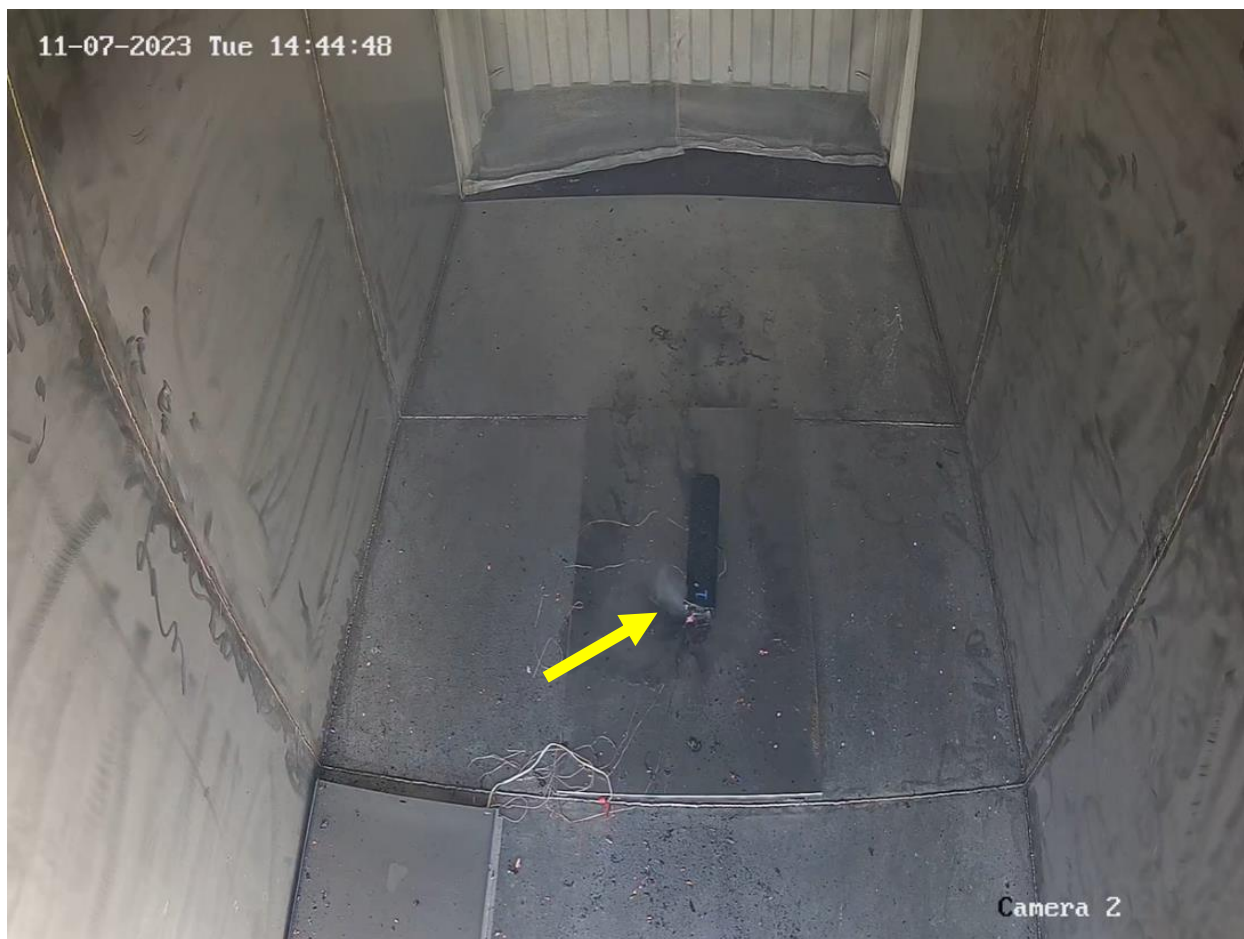
Figure 85. Small amount of smoke visible after application of FCL FSS (yellow arrow).
