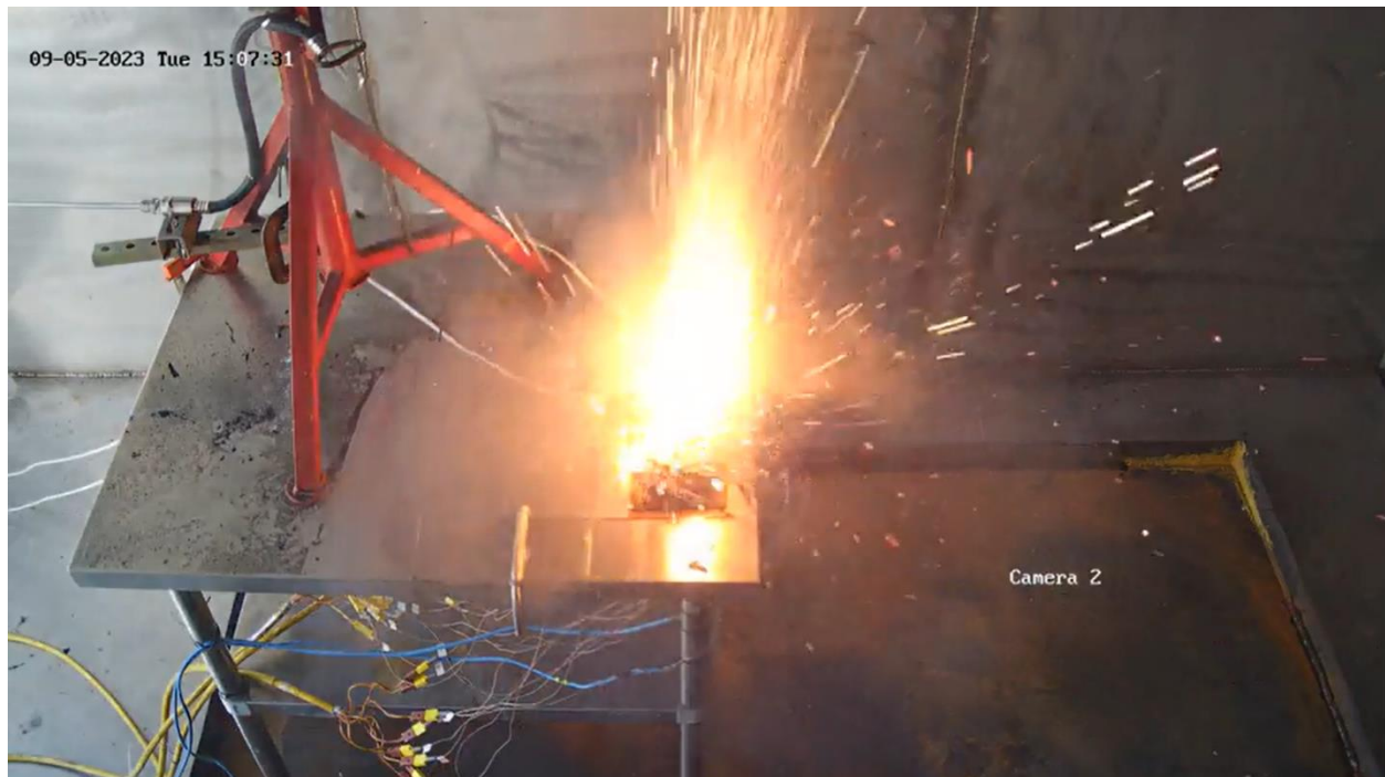
Figure 32. First cell experiencing thermal runaway in the control group.
