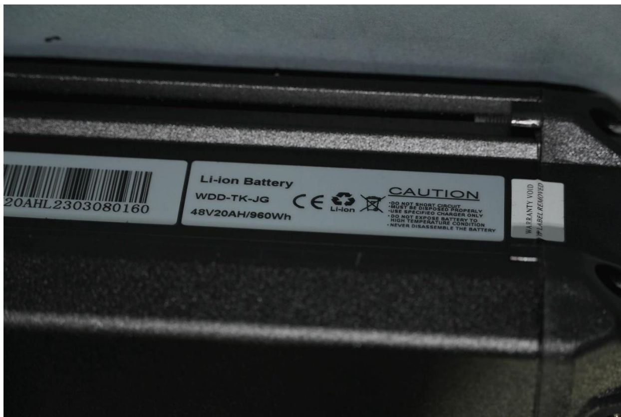
Figure 41. Bottom label of the E-Bike battery, 48V, 20 Ah, 960Wh.
