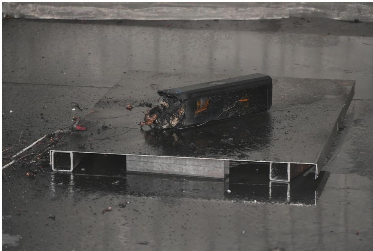
Figure 58. Photo of the E-Bike battery after third application of water.
