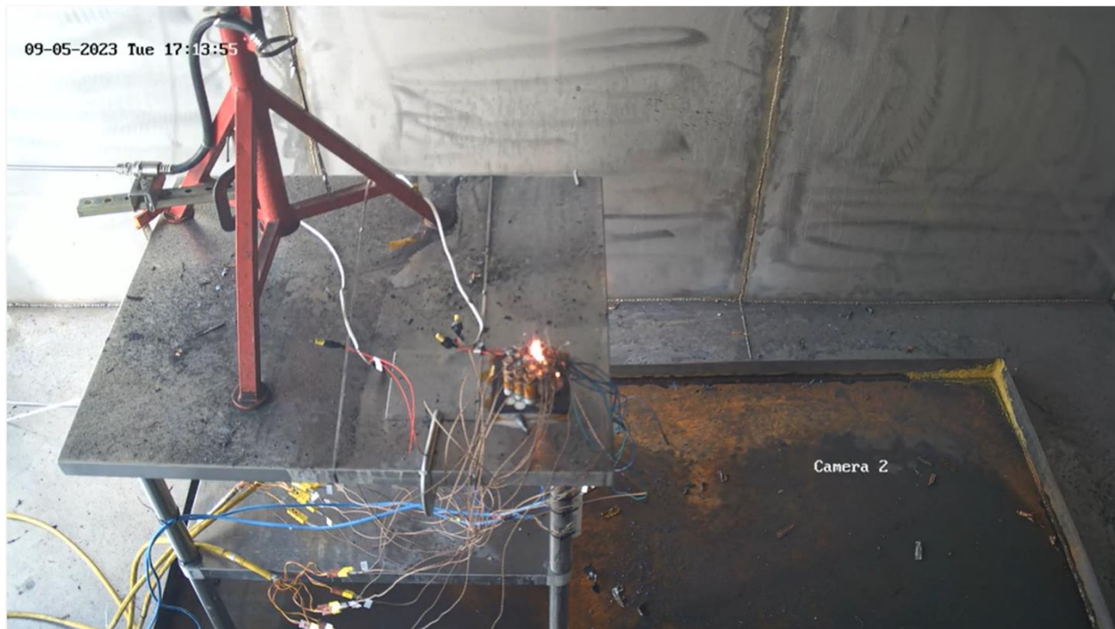
Figure 28. Several minutes after FSS was applied, a small flame appeared.
