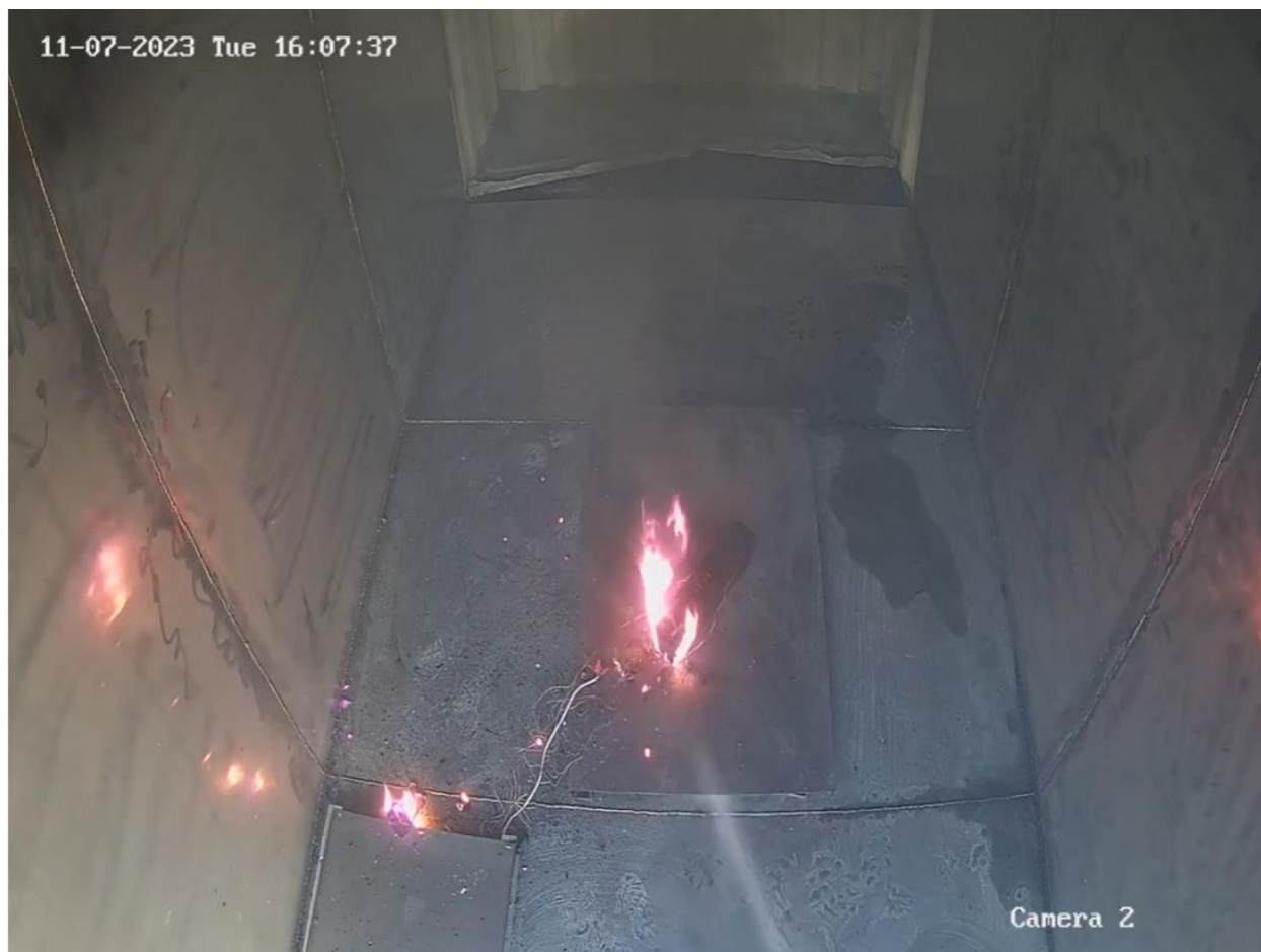
Figure 47. Water being applied to the battery.
